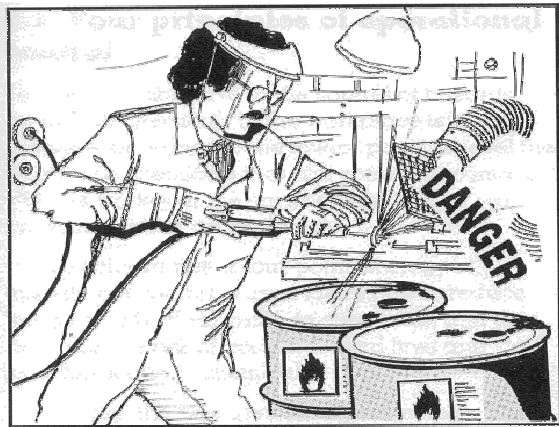
Figure 19. The open flame from welding and cutting torches can cause the ignition of flammable vapours
