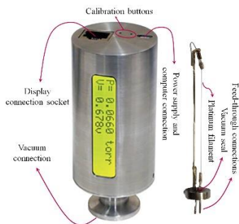
The fabricated Pirani vacuum gauge
