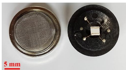
Photograph and SEM micrographs of a tin oxide methane sensor.
